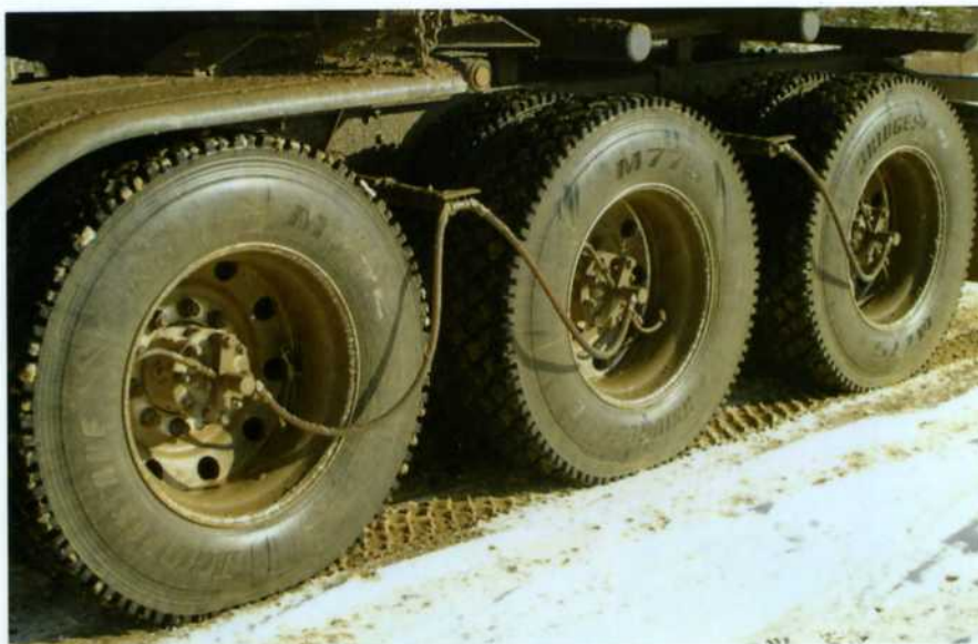
Tire pressure control helps keep this truck from getting stuck. The systems have also been used to dramatically reduce the amount of gravel required for logging roads.
